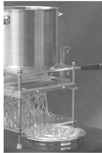
1. Remove the two crowned nuts on the front crossbar (circled in the picture) to expose the allen screws.
